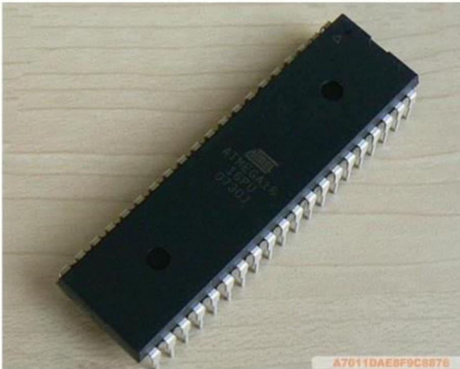
Fig : AVR Microcontroller
